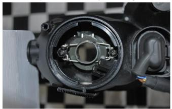
2. Plug in your headlight to the motorcycles wire harness and feed the wires and connector into the headlight housing. The driver (the rectangular box) will slide into the headlight housing. (Be patient. You may have to wiggle it around a bit to get it in there.) Once the driver is inside the housing, line up the keys and slide the bulb into the previously installed base. Give it a twist to the right to lock your new LED bulb into place.
